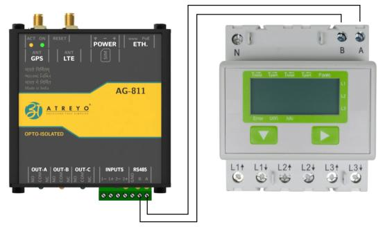
The device provide on-board  $120\Omega$  termination resistor for RS-485 port.
