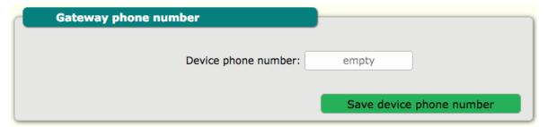
Cellular network testing is for testing of SIM card and network. You can add your number and Gateway will call or send SMS to this number. For this purpose, call and SMS support must be enabled with the mobile operator.
