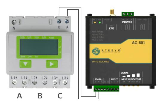
The device provide on-board  $120\Omega$  termination resistor for RS-485 port.
